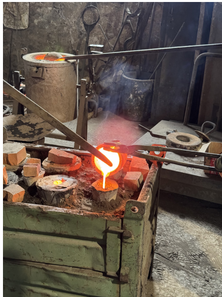
Figure 2 - Casting in the Marinelli Foundry of experimental replicas
